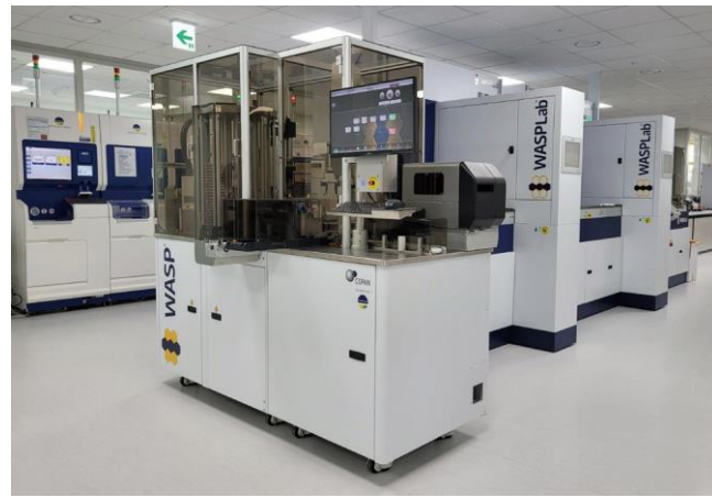
Fig. 1. Microbiology Laboratory TLA System (WASPLab®)
